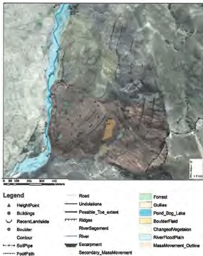
Figure 4: The layout of the Thendele rotational landslide imposed over a satellite image.
